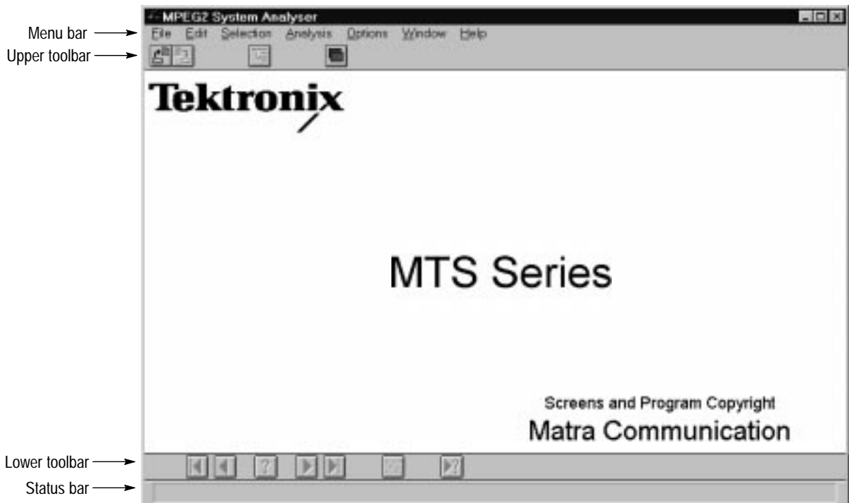
Figure 2-3: The Analyzer application window
